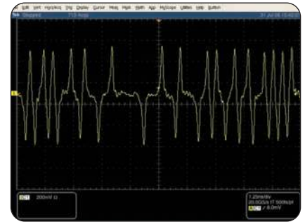
► Figure 3. Hard disk read channel signal (5 Gbps 2 points per cell); AWG7101 with 10 GS/s.
